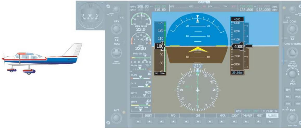
Figure 4-30. Pitch of the Aircraft.
