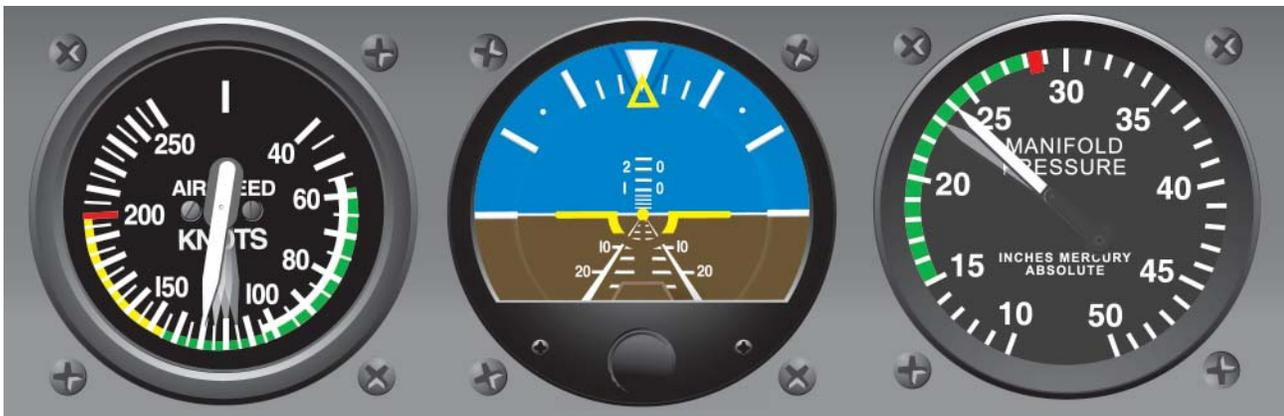
Figure 4-13. An Increase in Power Increasing Airspeed Accordingly in Level Flight.
