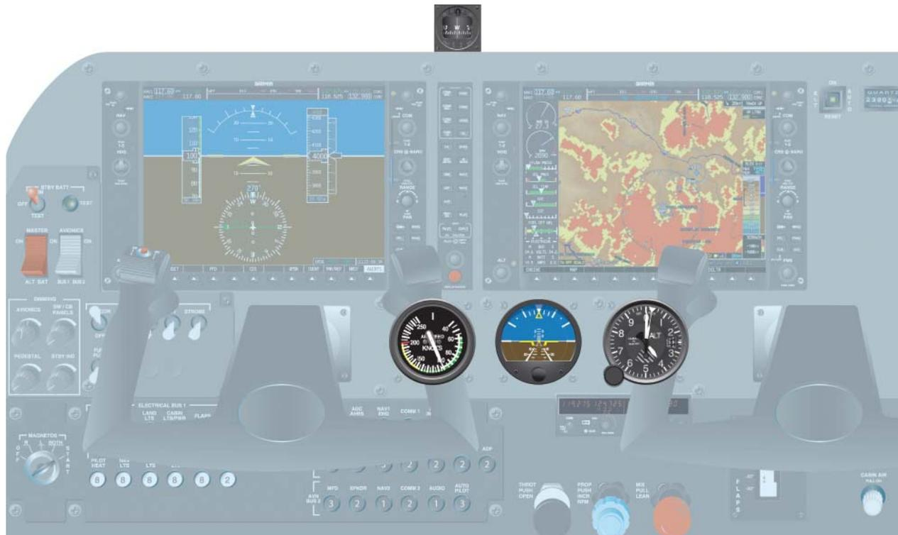
Figure 4-24. Emergency Back-up of the Airspeed Indicator, Attitude Indicator, and Altitude Indicator.
