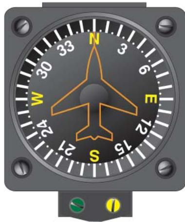
**Figure 3-22.** Vertical Card Magnetic Compass.
