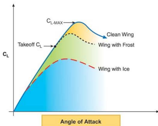
Figure 2-20. Effect of Ice and Frost on Lift.
