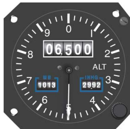
**Figure 3-5. Drum-Type Altimeter.**
