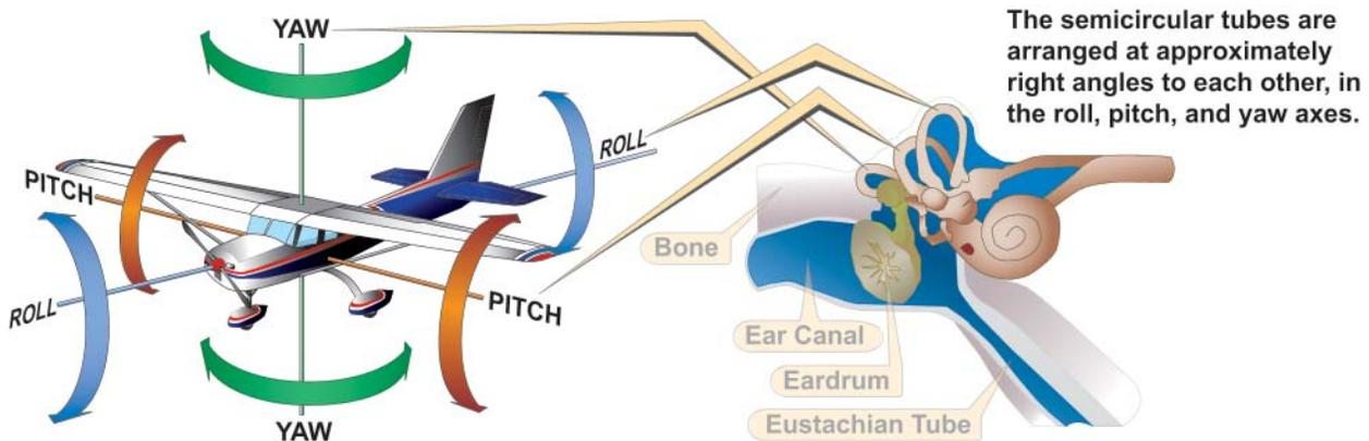
Figure 1-4. Angular Acceleration and the Semicircular Tubes.
