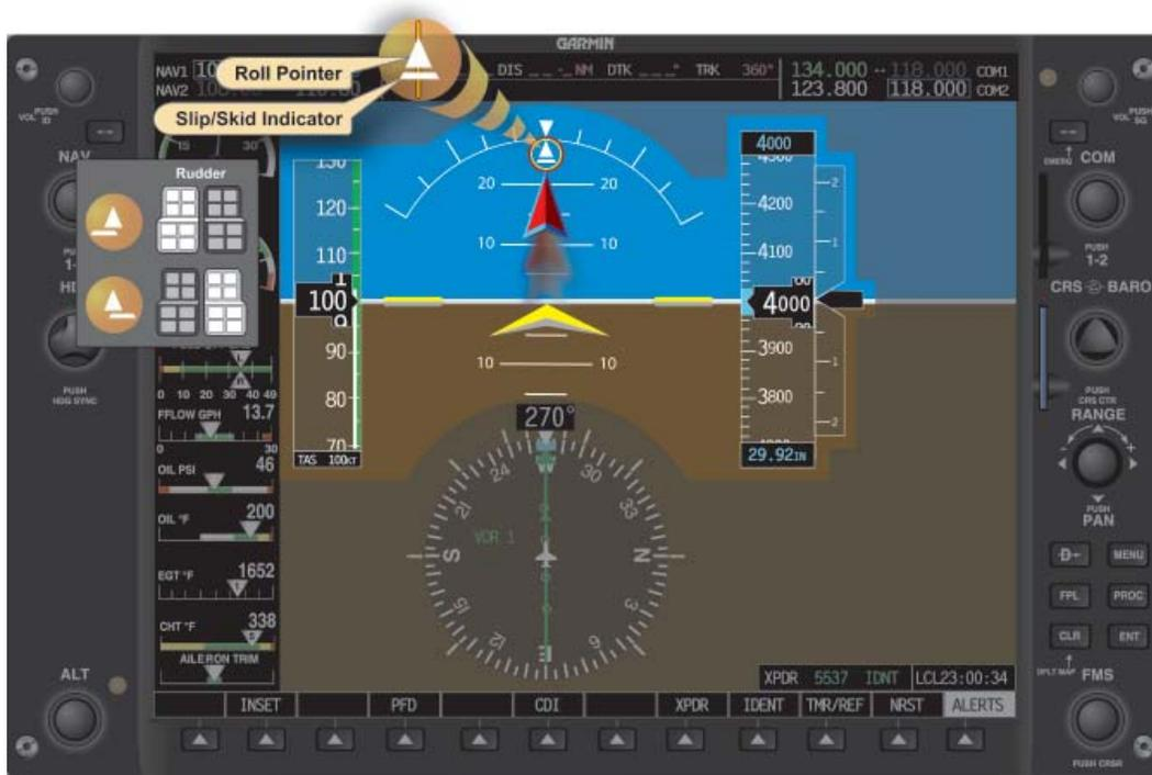
Figure 4-35. Roll Pointer and Slip/Skid Indicator.
