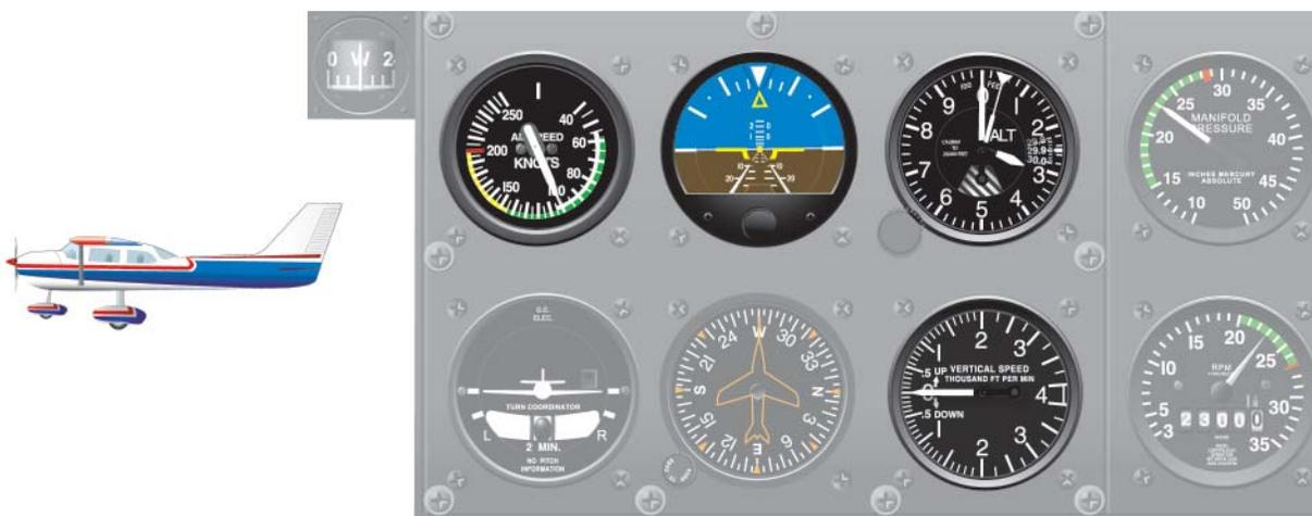
**Figure 4-4.** Pitch Instruments.
