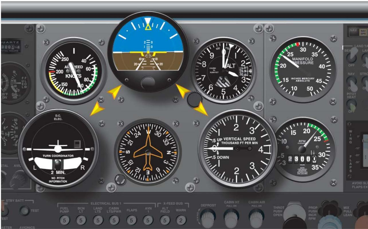
Figure 4-18. *Inverted-V Cross-Check.*
