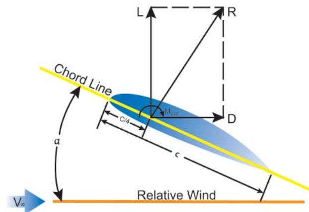
Figure 2-2. Angle of Attack and Relative Wind.
