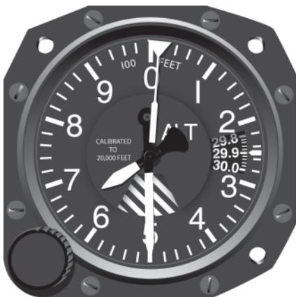
**Figure 3-4. Three-Pointer Altimeter.**
