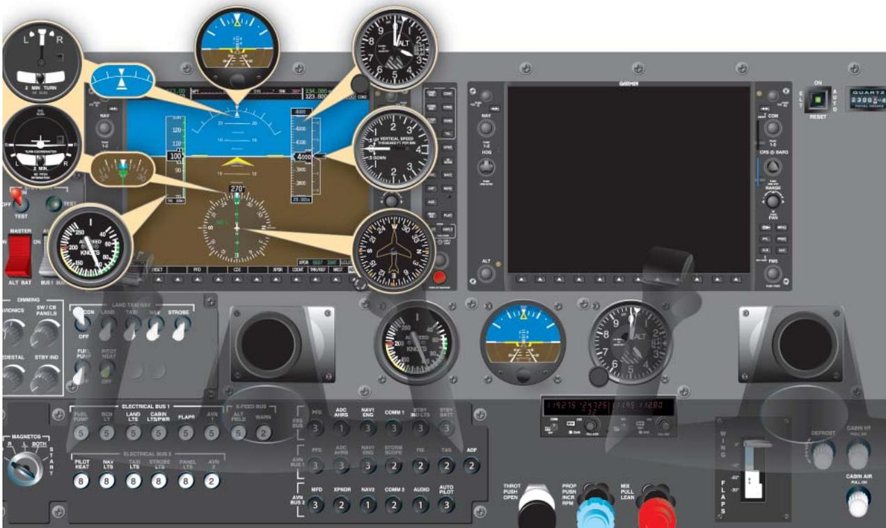
Figure 4-21. Primary Flight Display (PFD) and Analog Counterparts.
