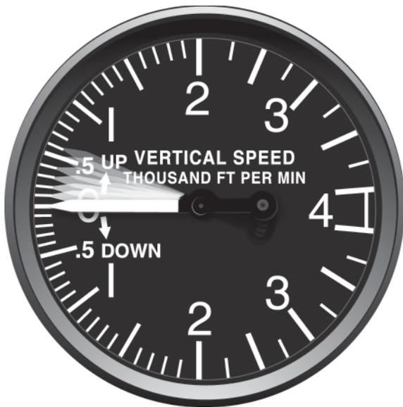
**Figure 4-8.** Vertical Speed Indicator.
