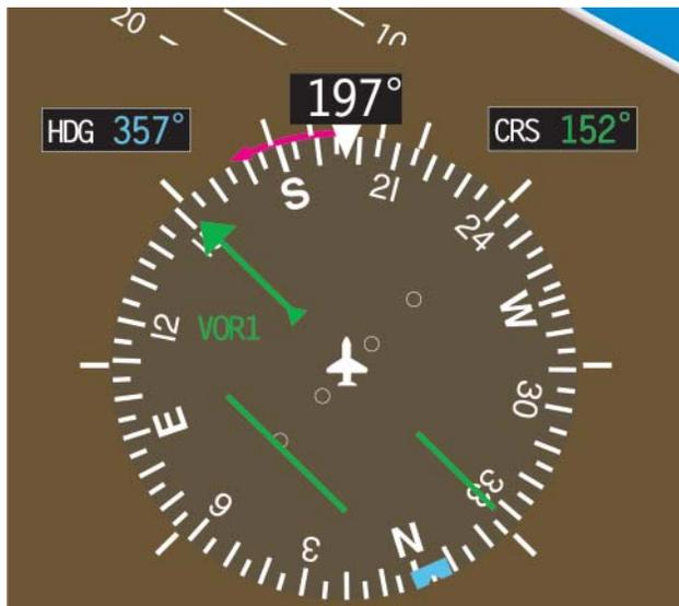
Figure 4-40. HSI Indicator (enlargement).
