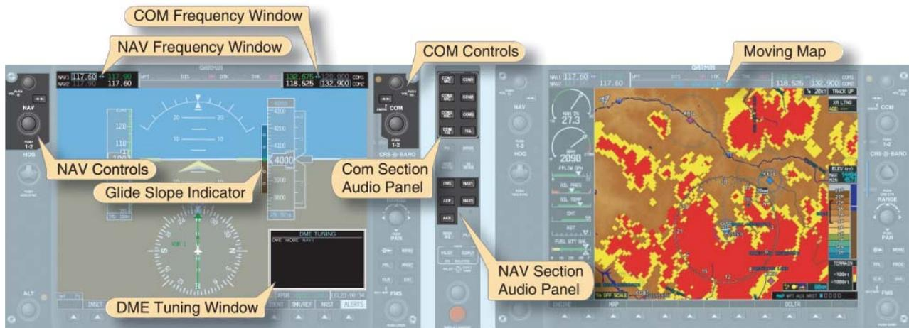
Figure 4-27. Navigation Instruments.
