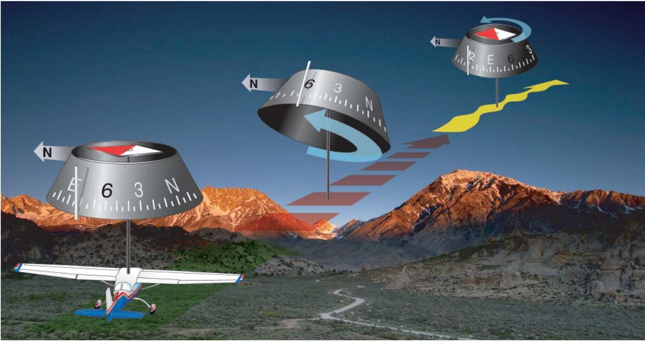
**Figure 3-21.** *The Effects of Acceleration Error.*
