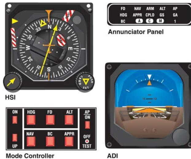
Figure 3-40. Components of a Typical Flight Director System.
