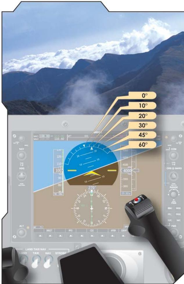
Figure 4-29. Bank Control Index Lines.
