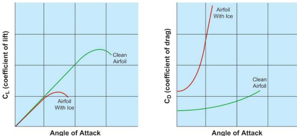
**Figure 2-19.** Aerodynamic Effects of Icing.
