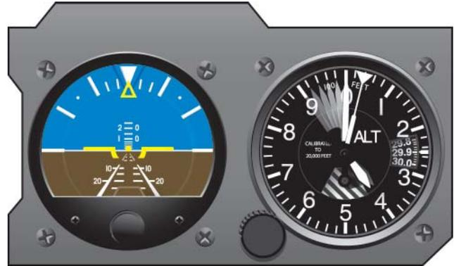
**Figure 4-6.** Pitch Correction Using the Attitude Indicator.
